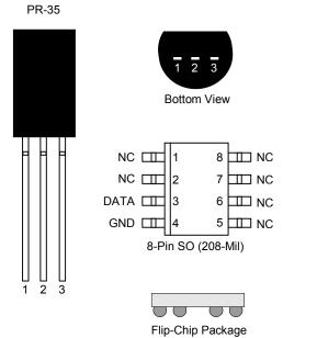
(Visit <u>www.maxim-ic.com</u> for flip-chip pinout and mechanical data.)
